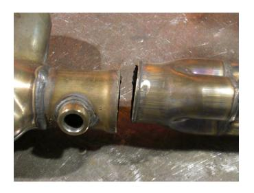
3. Grind cut area smooth around the outside. You also may need to do some clean up on the inside of the tube. Your new M4 unit slips not only over this area, but inside as well. We recommend checking your clean up job by taking the new unit and making sure it will slip on, and in, before you re-install the header unit.
