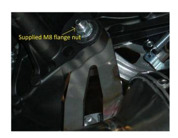
6. Check for clearance, tighten all mounting hardware, and re-attach your O2 sensor.
